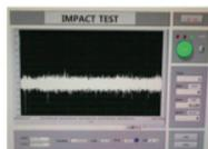
This test calculates the amount of impact the shock sensor receives at the bottom of the tester by dropping the impact weight at 1 meter height. By inserting the insert pieces on top of the sensor, you can see how much impact the insert absorbs.
